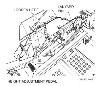
Figure 6-7. Cutter Deck Height Adjustment
